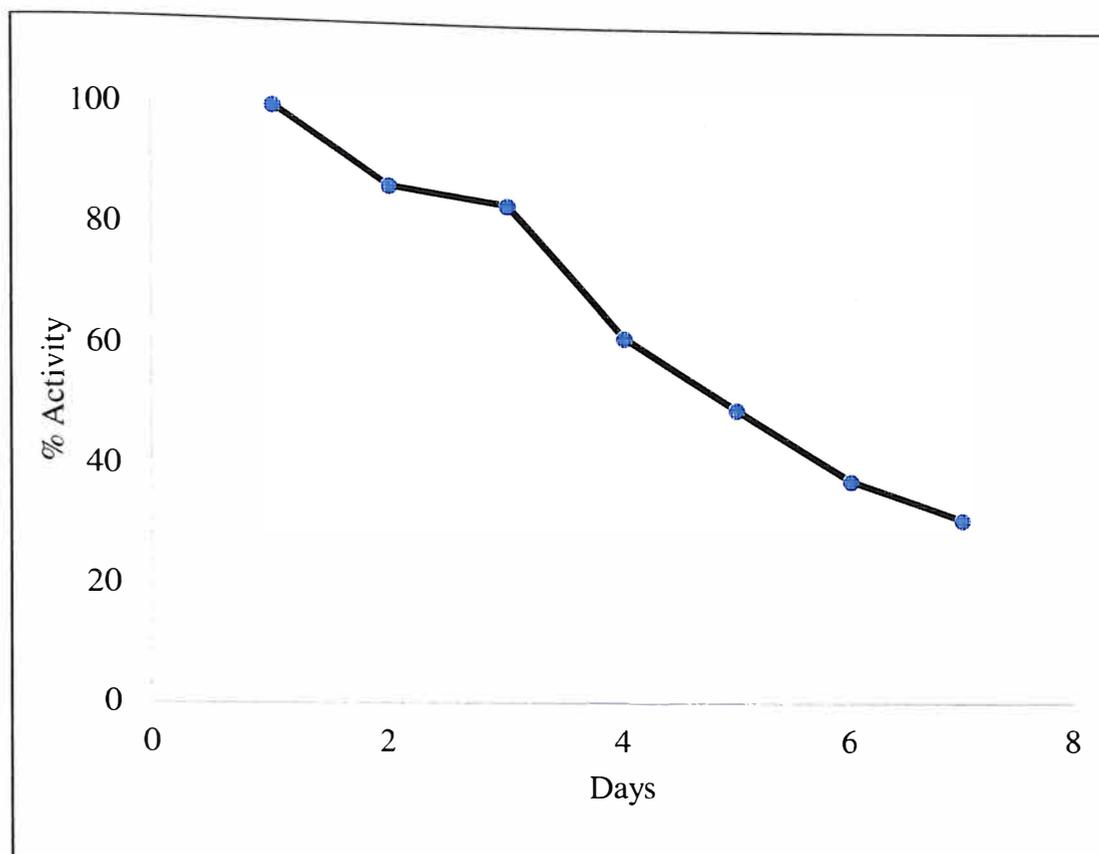
**Figure 4.10** % Activity of AuNPs/AchE/SPCE electrode as a function of days showing its shelf life.
