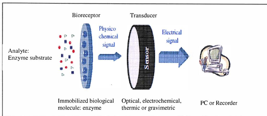
**Figure 2.5** Components of a biosensor.<sup>23</sup>
