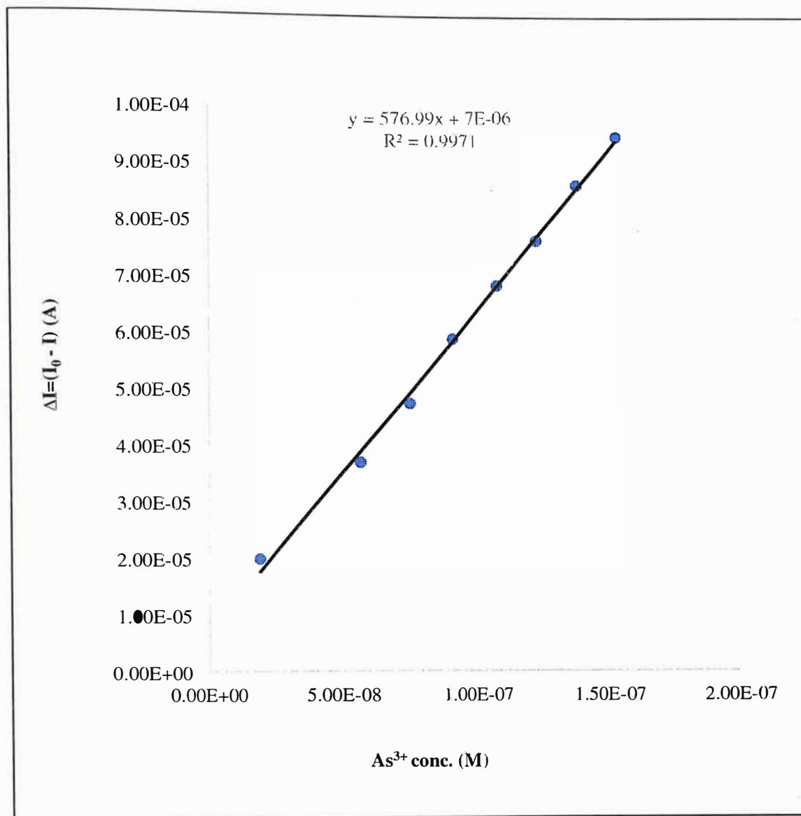
**Figure 4.5** Calibration plot of  $\Delta I$  vs.  $\text{As}^{3+}$  molar concentrations. Potential applied = +0.6 V vs. Ag/AgCl reference electrode using AchE/SPCE electrode in Britton-Robinson buffer pH = 7 and ATI concentration of  $3.64 \times 10^{-4}$  M
