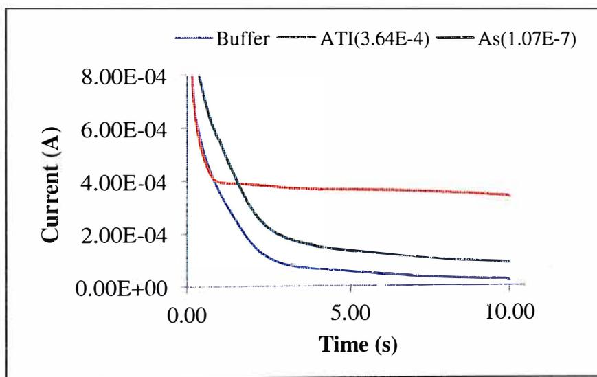
**Figure 4.3 (b)** Chronoamperogram obtained with AuNPs/AchE/SPCE electrodes at an applied potential of +0.6 V vs. Ag/AgCl reference electrode for Britton-Robinson buffer pH = 7,  $3.64 \times 10^{-4}$  M ATI, and  $1.07 \times 10^{-7}$  M  $\text{As}^{3+}$
