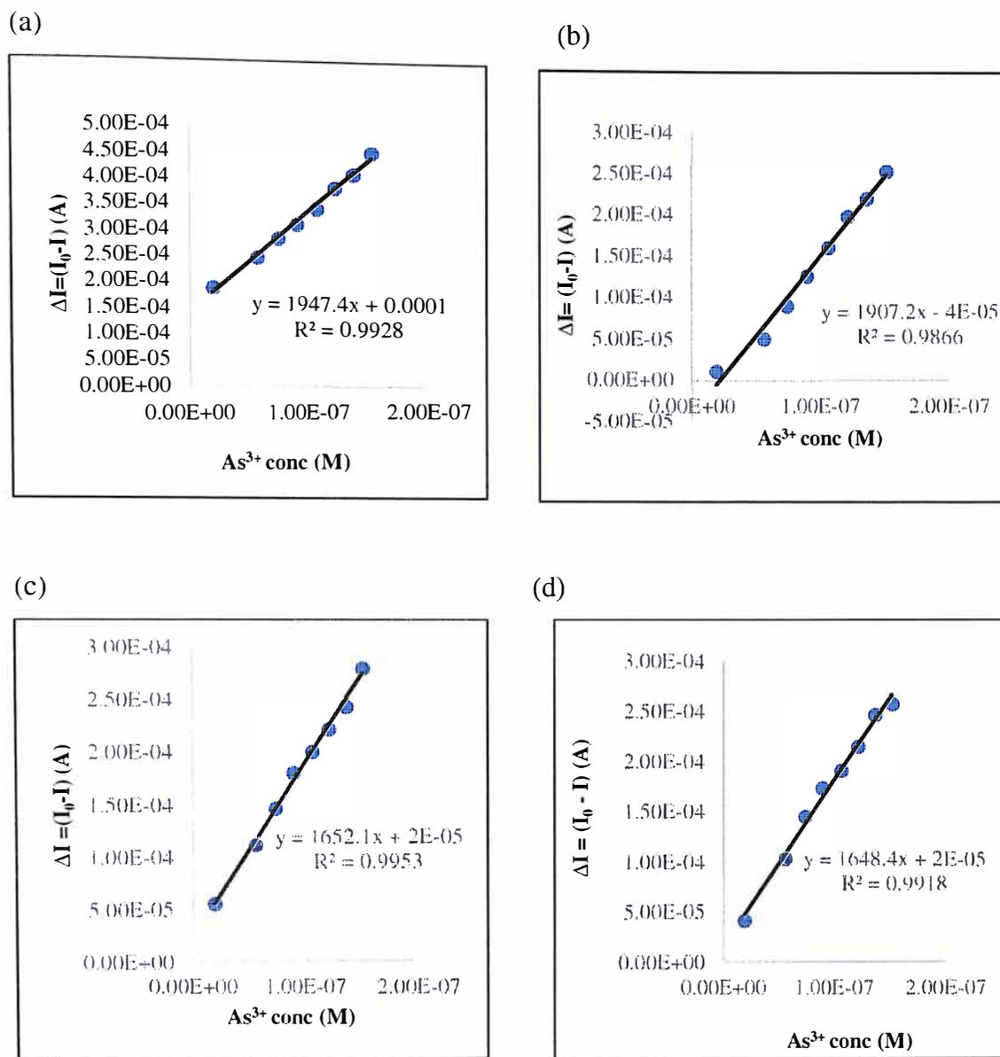
**Figure 4.8 (a) – (d)** Calibration plots of  $\Delta I$  vs.  $As^{3+}$  molar concentrations for the four sets of AuNPs/AchE/SPCEs. Potential applied = +0.6 V vs Ag/AgCl reference electrode in Britton-Robinson buffer pH = 7 and ATI concentration of  $3.64 \times 10^{-4}$  M
