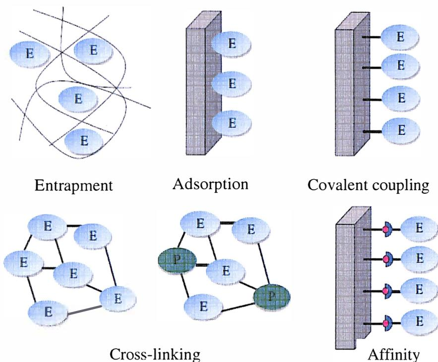
**Figure 2.6** Schematic representation of enzyme immobilization methods. E: enzyme, P: inert protein<sup>23</sup>
