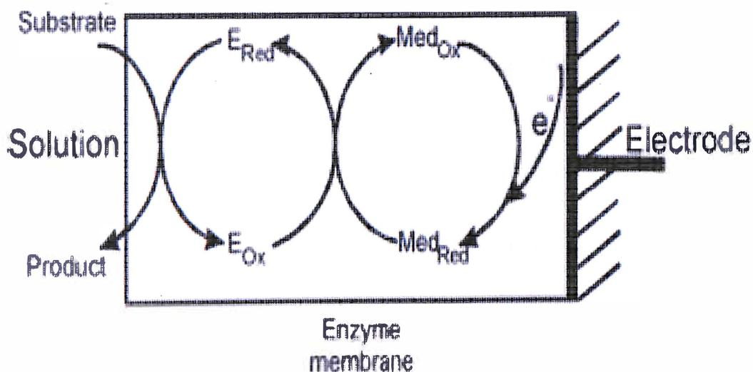
**Figure 2.7** Principle of operation of amperometric mediated biosensor.<sup>22</sup>
