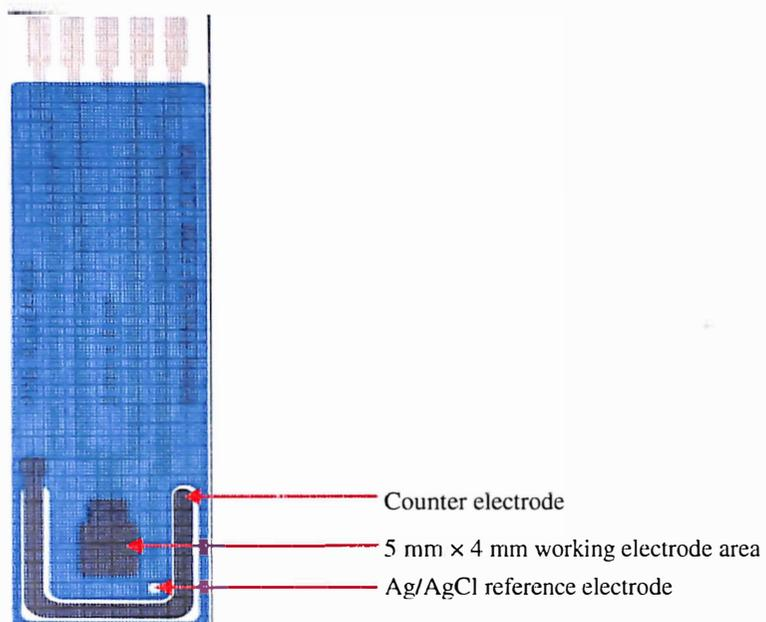
**Figure 3.2** screen printed carbon electrodes (SPCE)
