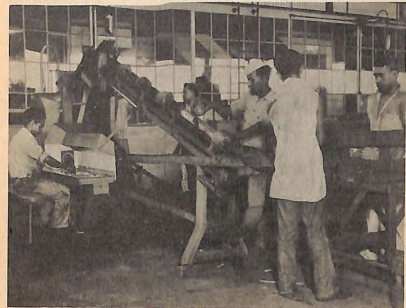
Feed Pineapples Into This Machine and They Come Out Cylinders Ready for the Slicing
