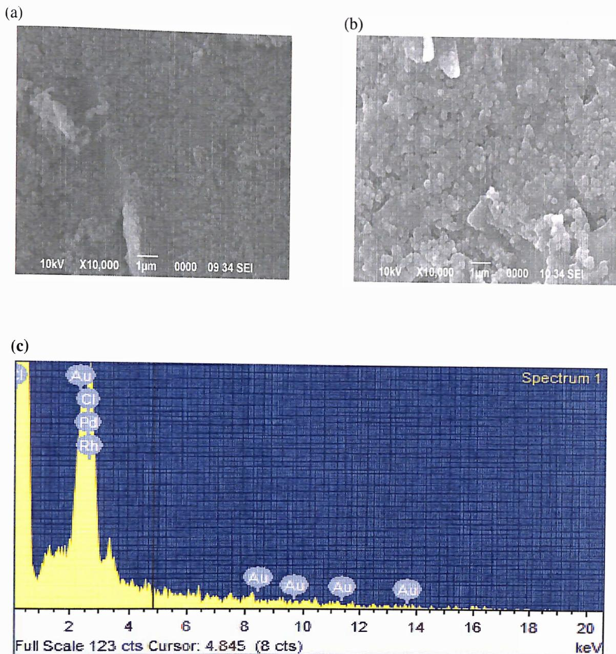
**Figure 4.2** (a) SEM micrograph of the working electrode bare SPCE. (b) SEM micrograph of the deposited film from a stirred solution of 0.1 mM gold (III) chloride trihydrate ( $\text{HAuCl}_4 \cdot 3\text{H}_2\text{O}$ ) in 0.5 M sulfuric acid by applying a potential of +0.18 V vs. Ag/AgCl for 15 s. (c) The EDS spectrum of the deposit in (b).
