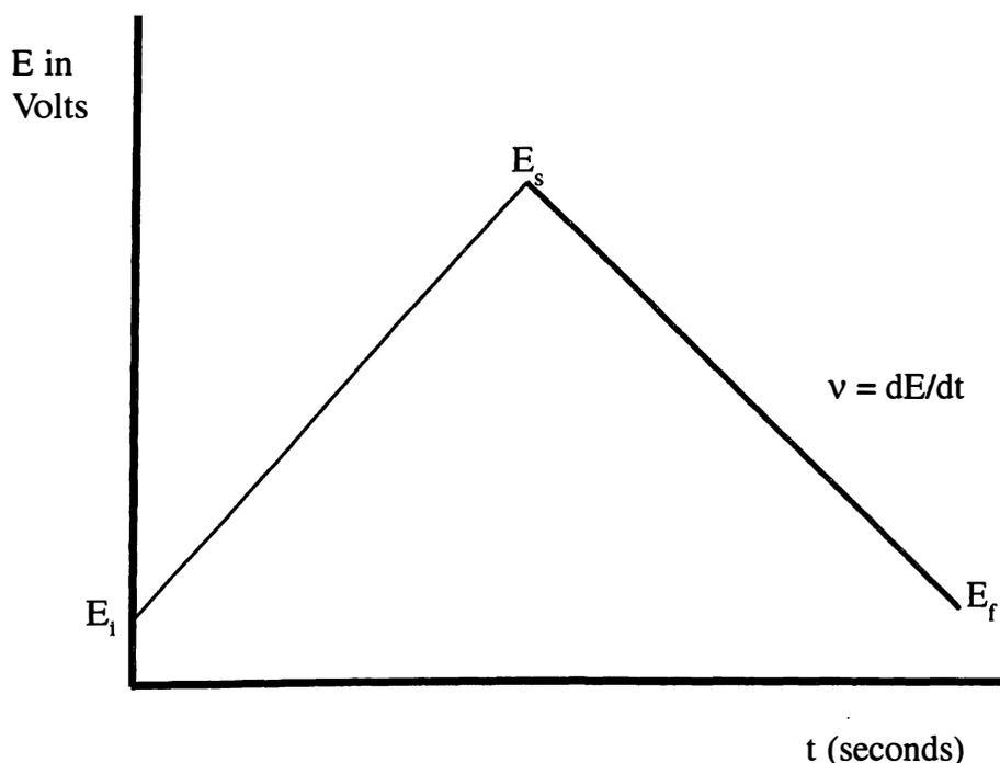
**Figure 2.9** Typical potential versus time signal for cyclic voltammetry.<sup>33</sup>
