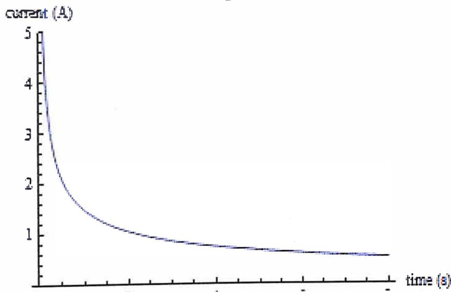
**Figure 2.11** (a) The potential-time profile for a single step chronoamperometric experiment. (b) Current vs. time response for a potential step experiment.  $E_2$  is chosen such that the reaction is diffusion controlled.
