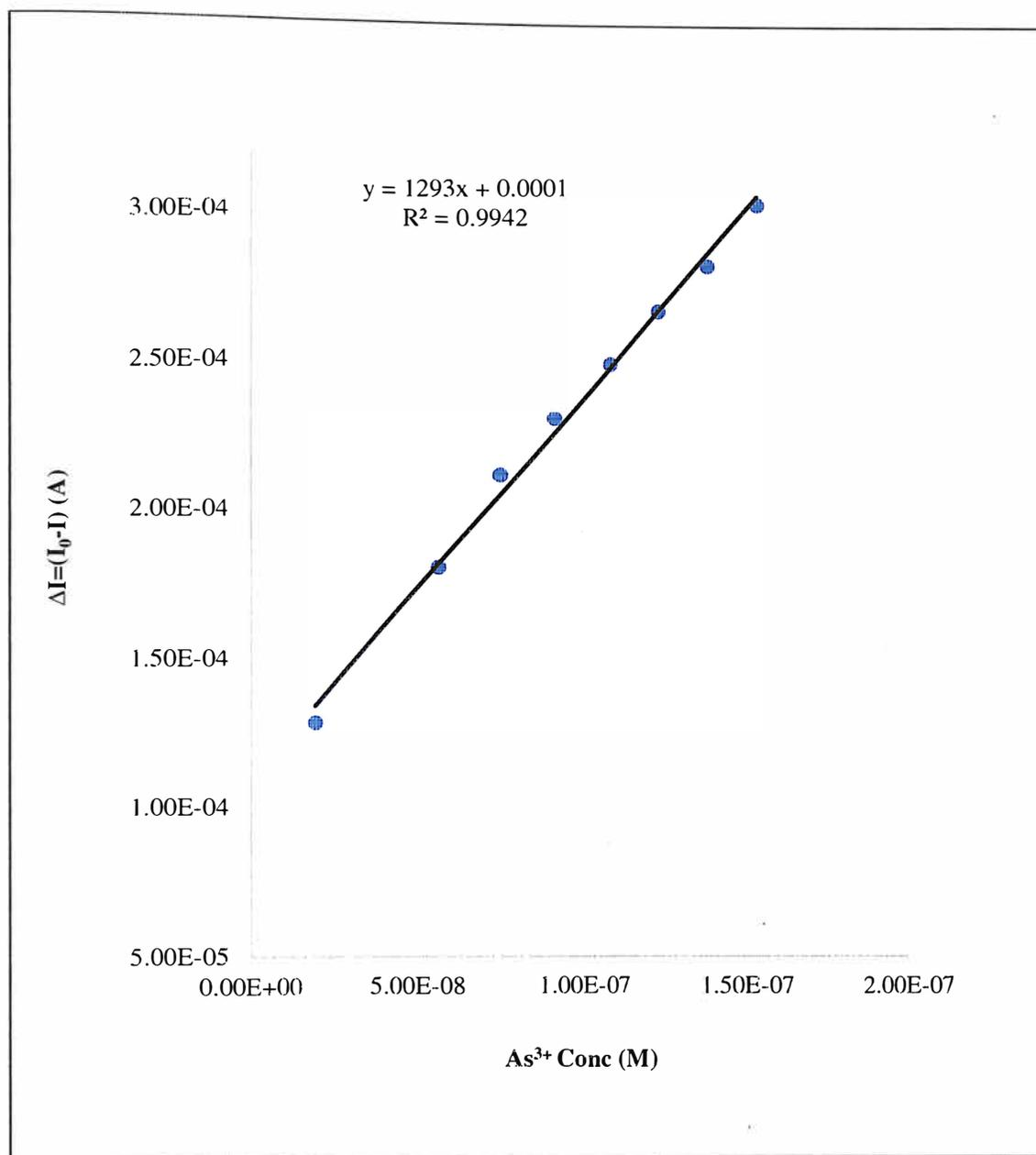
**Figure 4.7** Calibration plot of  $\Delta I$  vs.  $\text{As}^{3+}$  molar concentrations. Potential applied = +0.6 V vs. Ag/AgCl reference electrode using AuNPs/AchE/SPCE electrode in Britton-Robinson buffer pH = 7 and ATI concentration of  $3.64 \times 10^{-4}$  M
