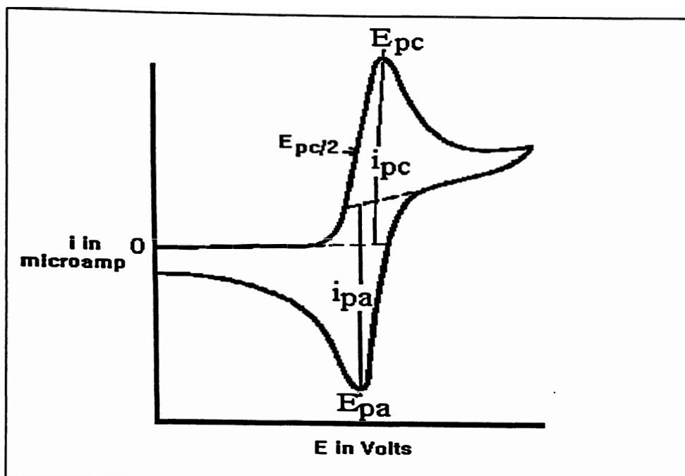
**Figure 2.10** Typical cyclic voltammetric output for a reversible redox couple.  $E_{pc}$  and  $E_{pa}$  represent the cathodic and anodic peak potentials, respectively. The cathodic and anodic peak currents are represented by  $i_{pc}$  and  $i_{pa}$ , respectively.<sup>34</sup>
