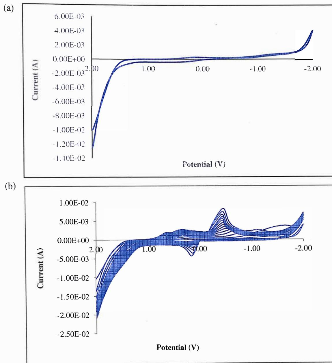
**Figure 4.1** Cyclic voltammograms during activation of the SPCE in 0.1 M KCl: (a) for the first scan and (b) for multiple scans. Potential were recorded vs. Ag/AgCl reference electrode.
