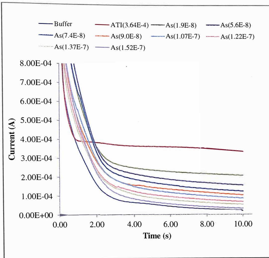
**Figure 4.6** Chronoamperogram obtained with AuNPs/AchE/SPCE electrode at an applied potential of +0.6 V vs. Ag/AgCl reference electrode for Britton-Robinson buffer pH = 7,  $3.64 \times 10^{-4}$  M ATI, and various molar concentrations of As<sup>3+</sup> shown in parenthesis.
