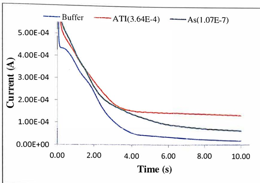
**Figure 4.3 (a)** Chronoamperogram obtained with AchE/SPCE electrodes at an applied potential of +0.6 V vs. Ag/AgCl reference electrode for Britton-Robinson buffer pH = 7,  $3.64 \times 10^{-4}$  M ATI, and  $1.07 \times 10^{-7}$  M  $\text{As}^{3+}$
