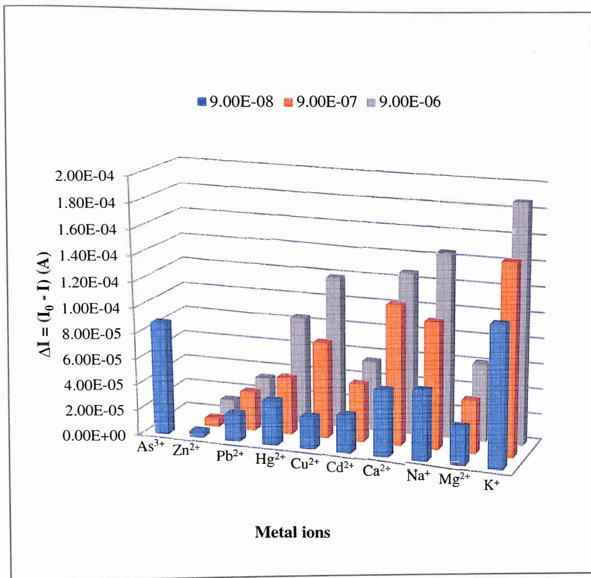
**Figure 4.9** Inhibition current of metals ions on AuNPs/AchE/SPCE electrode in presence of As<sup>3+</sup> solution at  $9.00 \times 10^{-8}$  M.
