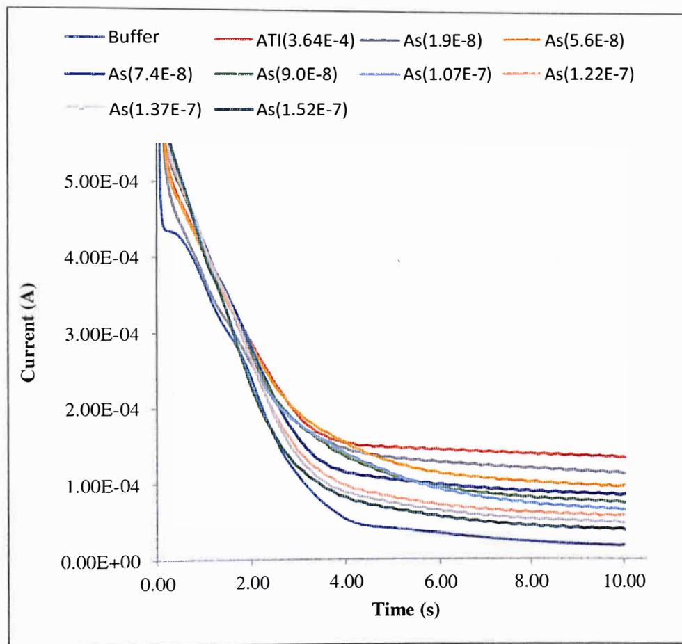
**Figure 4.4** Chronoamperograms obtained with AchE/SPCE electrodes at an applied potential of +0.6 V vs. Ag/AgCl reference electrode for Britton-Robinson buffer pH = 7,  $3.64 \times 10^{-4}$  M ATI, and various molar concentrations of  $\text{As}^{3+}$  shown in parenthesis.
