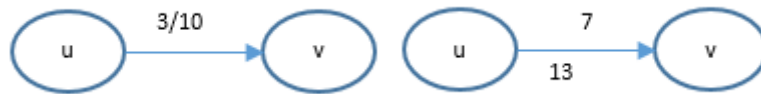
Figure 2 : Example graph G = \{u, v\}, \{e\} consisting of two nodes u, v and one edge e [20]. e has (undirected) capacity 10 and the flow on it is f(u, v) = 3 . Left: Flow network. The diamond shaped arrowhead of the edge indicates flow direction. Right: Corresponding residual flow network. In the residual network, the edge from u to v has residual capacity 10 - 3 = 7 , and c_f(v, u) = 10 - (-3) = 13 .
